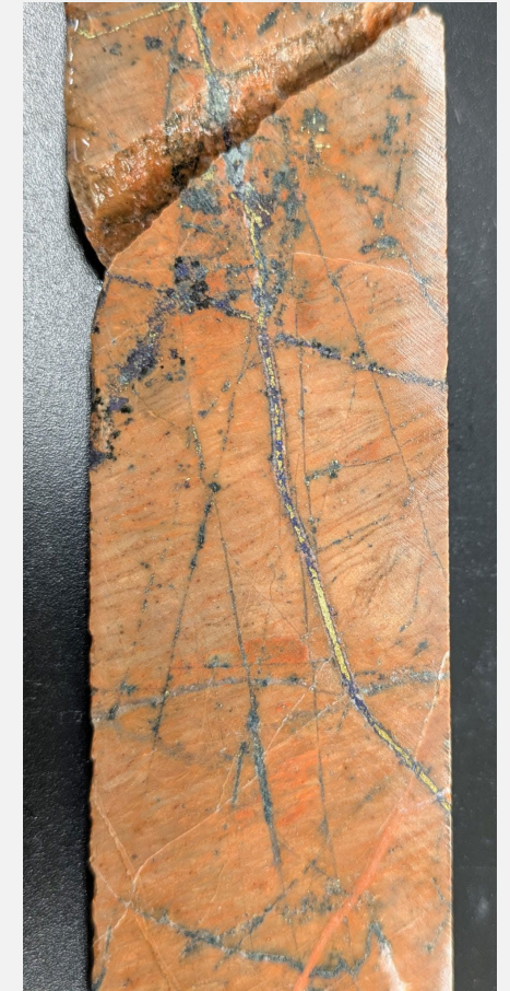
MEPS-25-02 GFP grading 0.85% Cu, 0.054 g/t Au and 7.1 g/t Ag over 0.8m
