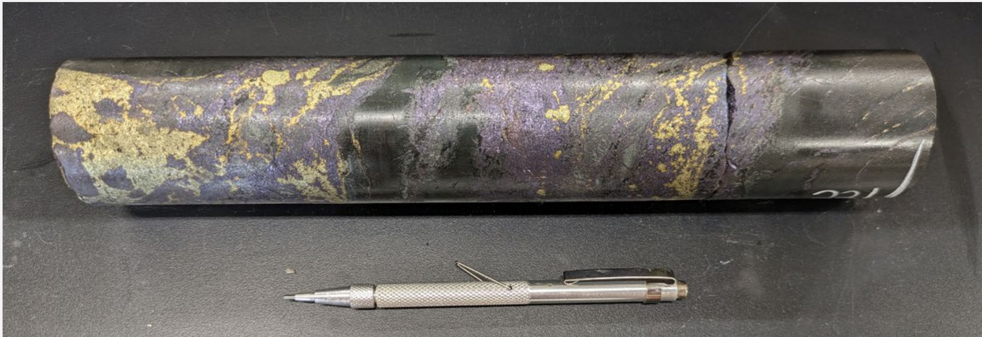
MEPS-25-02 grading 33% Cu, 0.342 g/t Au and 210 g/t Ag over 0.55m
