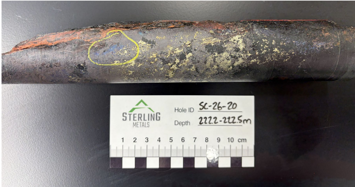
Figure 3. SC-26-20 at approximately 222.2m depth. Semi-massive magnetite with chalcopyrite and covellite (circled in yellow), illustrating the local association between stronger copper grades and magnetite. Sample interval 221.90m to 222.75m returned 0.85m grading 5.42% CuEq (4.74% Cu, 0.531 g/t Au, 17.7 g/t Ag and 19 ppm Mo).
