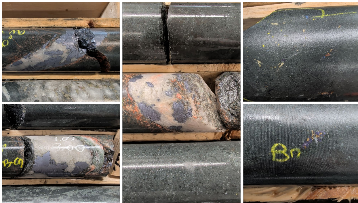
Figure 5. Robust molybdenite and chalcopyrite veining with traces of bornite and covellite in hole SC-26-19 from 216m depth to 247m depth
