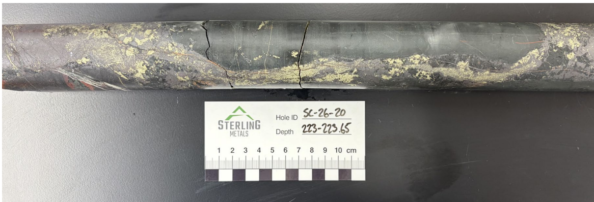
Figure 4. SC-26-20 at approximately 223m depth. Semi-massive magnetite with chalcopyrite. Sample interval 222.75m to 223.65m returned 0.90m grading 4.53% CuEq (3.64% Cu, 0.557 g/t Au, 34.8 g/t Ag and 20 ppm Mo).
