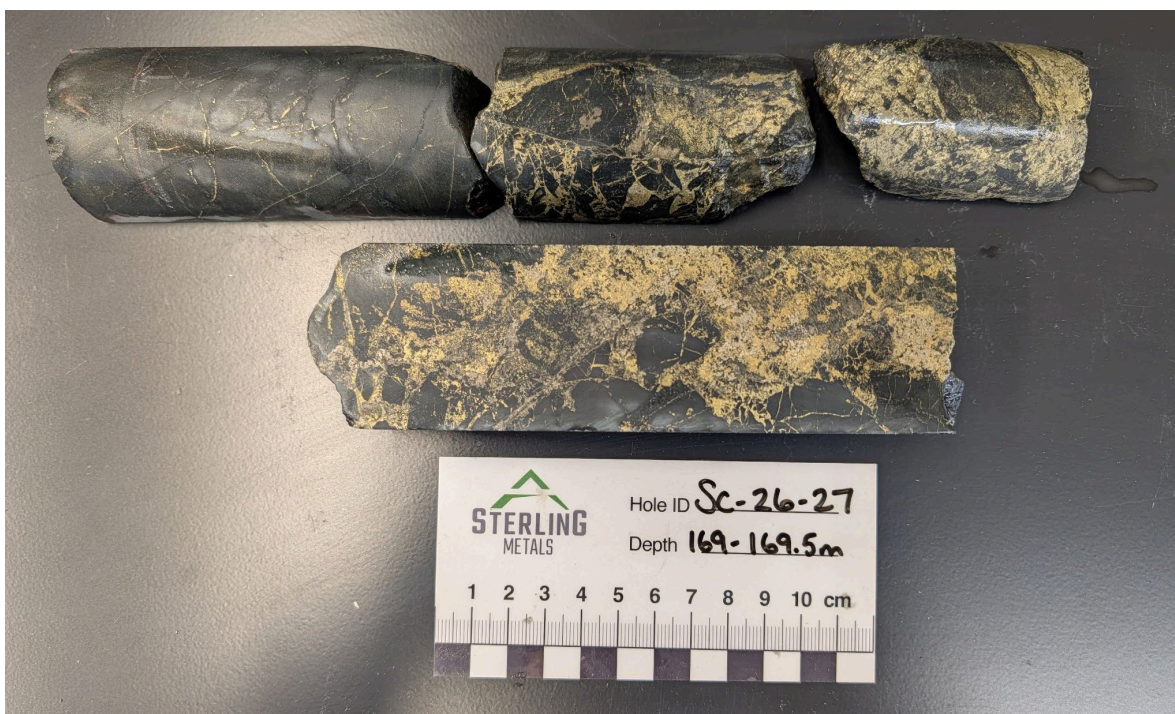
Figure 4. High-grade, high-tenor copper sulphide (chalcopyrite) mineralization in hole SC-26-27 from 169.00m to 169.50m depth grading 6.65% CuEq (6.36% Cu). Copper-rich mineralization in association with strong hydrothermal breccia development.
