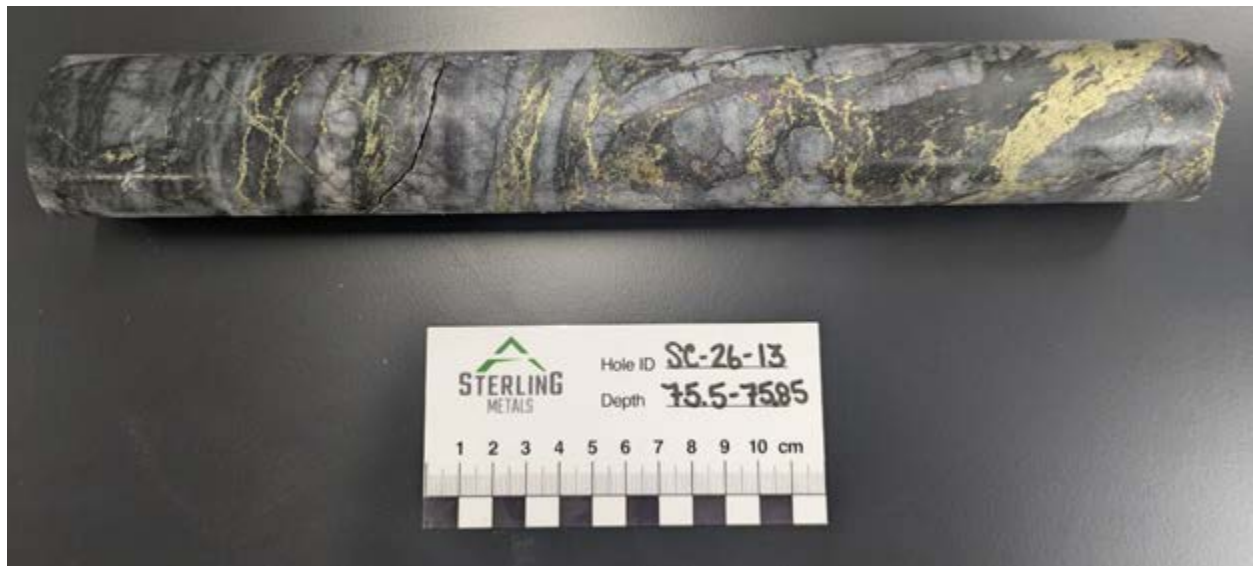
Figure 3. Chalcopyrite- and bornite-rich ribbon vein in SC-26-13 at approximately 75.5 m downhole. The sample returned 10.8% Cu, 16.6 g/t Au, 145 g/t Ag and 10 ppm Mo
