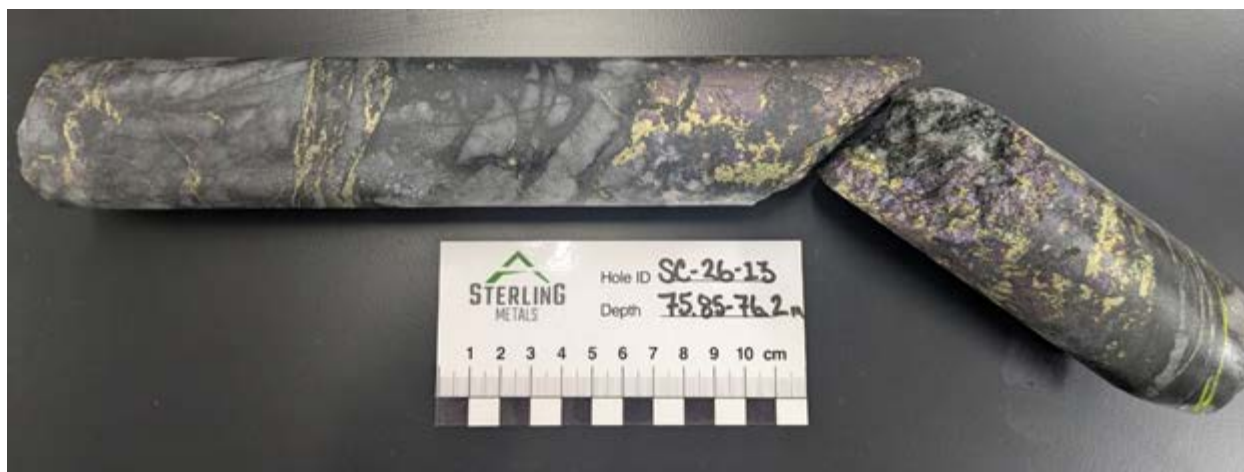
Figure 4. Chalcopyrite- and bornite-rich ribbon vein in SC-26-13 at approximately 75.85 m downhole. The 0.35-m sample returned 11.7% Cu, 2.63 g/t Au, 198 g/t Ag and 52 ppm Mo.
