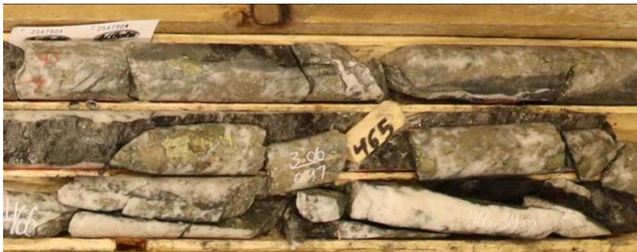
Figure 6. Chalcopyrite-rich quartz breccia in SC-26-13 at approximately 465 m downhole within a 7.4m interval grading 1.13% Cu, 0.076g/t Au, 14.8g/t Ag and 259.5ppm Mo
