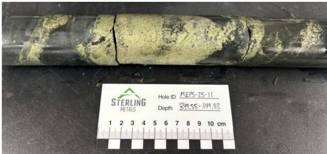
Figure 4. Massive chalcopyrite mineralization in MEPS-25-11 at 349.55m grading 13.1% Cu, 0.2 g/t Au, 22 g/t Ag and 340 ppm Mo
