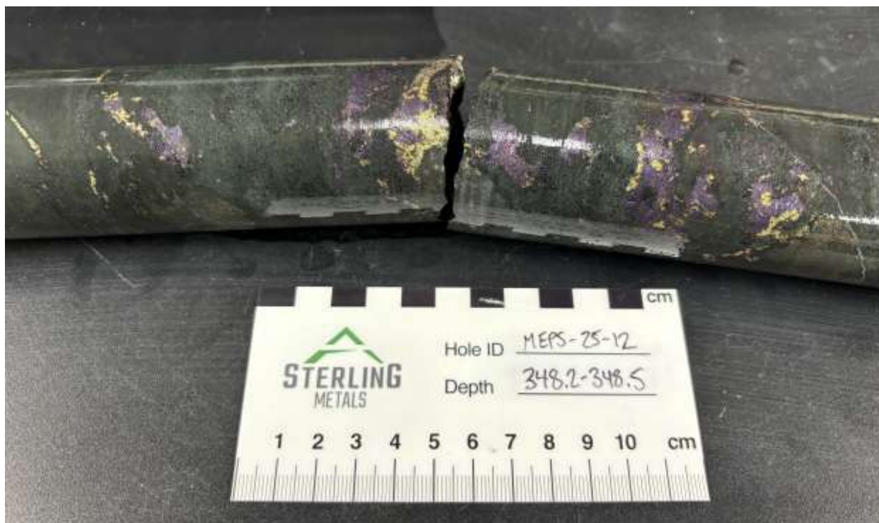
Figure 5. Bornite and chalcopyrite mineralization in MEPS-25-12 at 348.2m grading 8.2% Cu, 4.86 g/t Au, 71.4 g/t Ag and 20 ppm Mo
