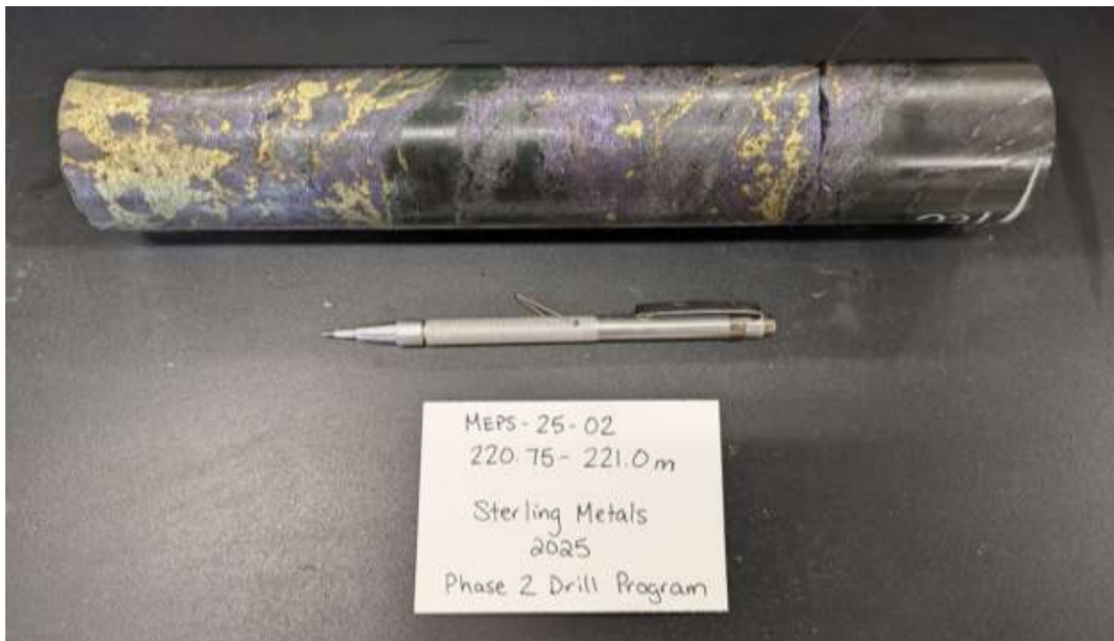
Figure 2. Bornite-chalcopyrite mineralization at 220.75m depth in MEPS-25-02 grading 33% Cu, 0.342 g/t Au and 210 g/t Ag over 0.55m.
