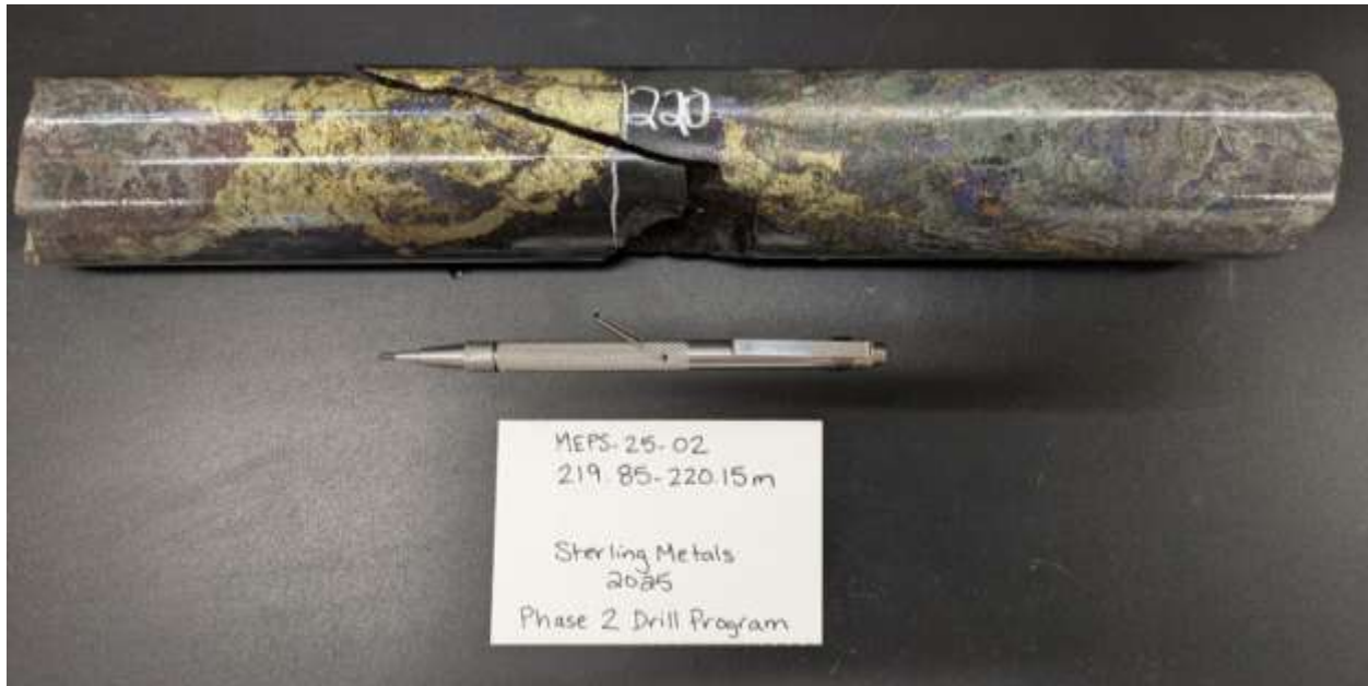
Figure 1. Bornite, chalcopyrite and gold mineralization in MEPS-25-02 at 219.85m depth grading 23.1% Cu, 196 g/t Au and 168 g/t Ag over 0.6m.
