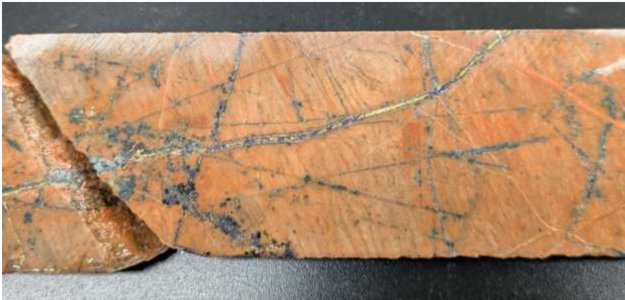
Figure 4. Chalcopyrite and bornite copper mineralization in GFP porphyry unit in MEPS-25-02 at 216.2m depth grading 0.847% Cu, 0.054g/t Au and 7.1g/t Ag
