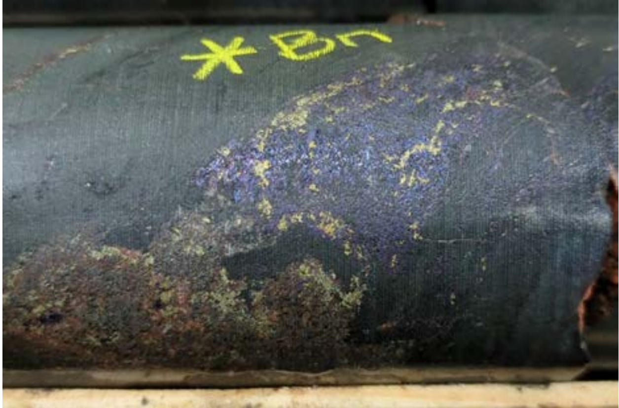
Figure 5. Bornite-chalcopyrite mineralization at 264.9m depth in MJ-25-01 grading 2.95% Cu, 0.442 g/t Au and 24 g/t Ag over 0.6m. Hosted by strongly biotite-chlorite altered mafic tuff volcanics adjacent to early stage GFP Porphyry.
