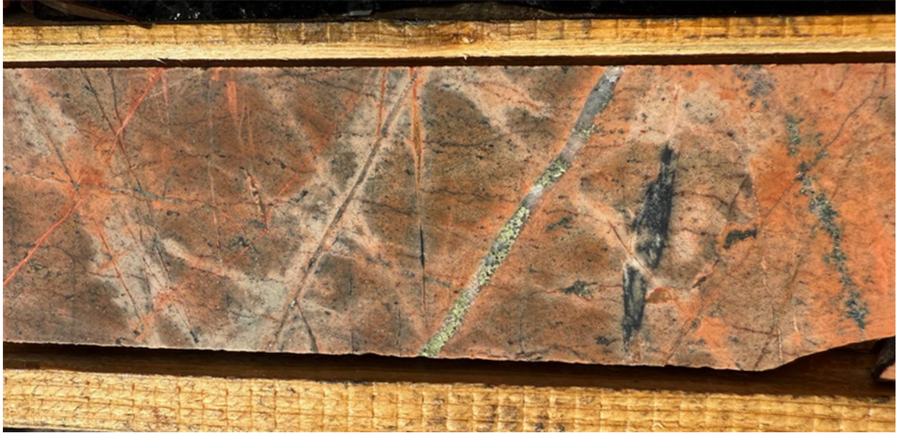
Figure 6. Intensely veined and newly discovered, early stage GFP Porphyry at 267m depth grading 0.68% Cu, 0.02% Mo, 0.19 g/t Au and 4.2 g/t Ag. Split NQ core (4.8cm wide).
