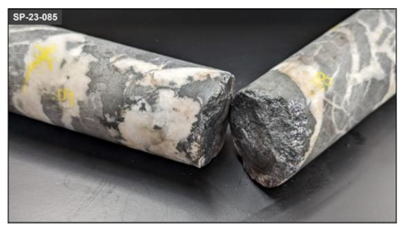
Figure 5. Drill core photo of high-grade mineralization in hole SP-23-085 from 208.97m to 209.29m
