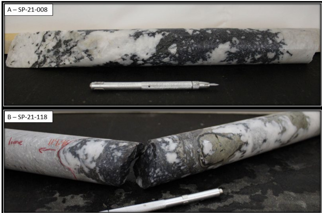
Figure 1: Drill core from the South Zone of the Sail Pond Project. A: Quartz-vein hosted sulfide and sulfosalt mineralization, including tetrahedrite-tennantite, galena, and sphalerite at 174.55 m in hole SP-21-008. The sample returned 1039.63 g/t AgEq comprised of 320.00 g/t Ag, 0.08 g/t Au, 0.79 % Cu, 15.10 % Pb, 0.25 % Sb, & 1.66% Zn over 0.55 metres. B: Quartz-vein hosted sulfide and sulfosalt mineralization, including tetrahedrite-tennantite, sphalerite, galena, and chalcocite at 114.45 m in hole SP-21-018. The sample returned 1,854.02 g/t AgEq comprised of 612 g/t Ag, 0.2 g/t Au, 2.26 % Cu, 3.35 % Pb, 0.86 % Sb, & 14.7 % Zn over 0.4 metres
